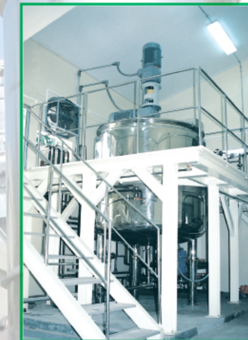
SHAMPOO / CONDITIONER / LOTION MIXING TANK 3,500L (OPEN TYPE)
